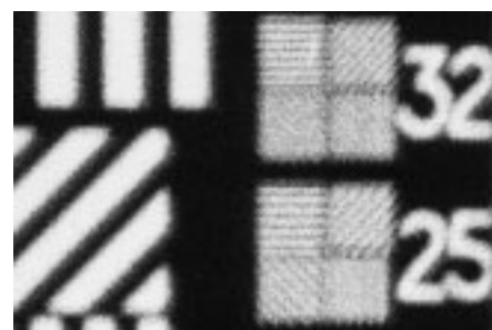
Film displaced only 0.3 \text{ mm} ( 1/80'' ) from the optimum image plane (at full aperture).
